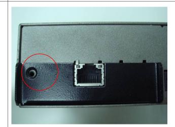
12. When correctly inserted, there is a screw hole at the upper left hand corner.
