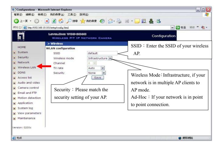
Please press "save" after configuration, and then unplug your power cord and RJ-45 LAN cable. Insert Power cord in; do not insert RJ-45 LAN cable. LevelOne IP camera should automatically connect to the preset AP.
