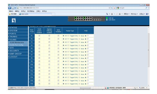
9. Now you may test the isolation between VLAN 2 and VLAN 3. And also the access to internet via the gateway connected on port 1.
