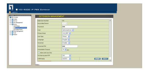
When finishing configuration, you will need to click on Reload button under Service --> IP PBX service in order to save the setting.
