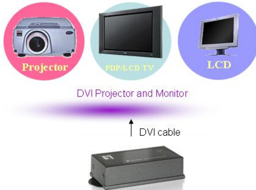
Connect ADE-8002 to DVI Monitor by DVI Cable
