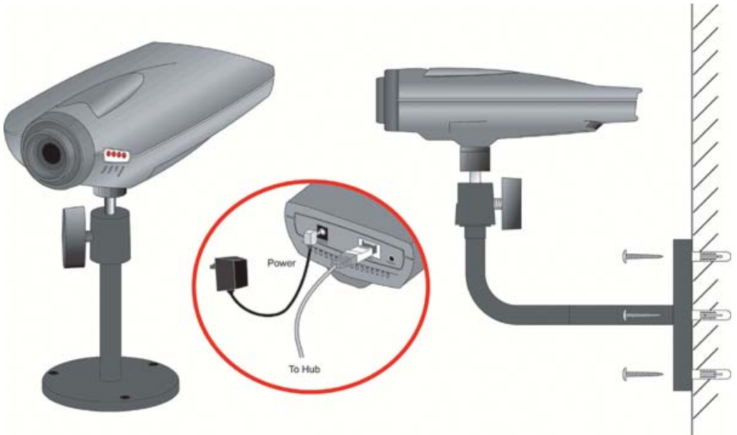
Figure 3: LevelOne IP Network Camera Installation
