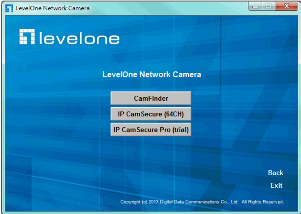
“Cam Finder” is used to search the IP address of Network Cameras or Video servers on a LAN. After searching, Video Servers or Network Cameras will be located by the Cam Finder.
