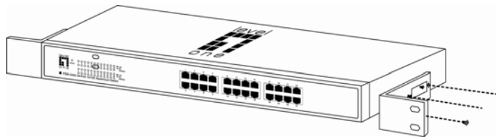
Figure 2-1 Rivet the 'L'brackets onto the Switch
