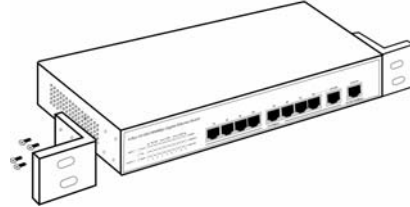
Figure 2- 2A. Attaching the mounting brackets to the Switch
