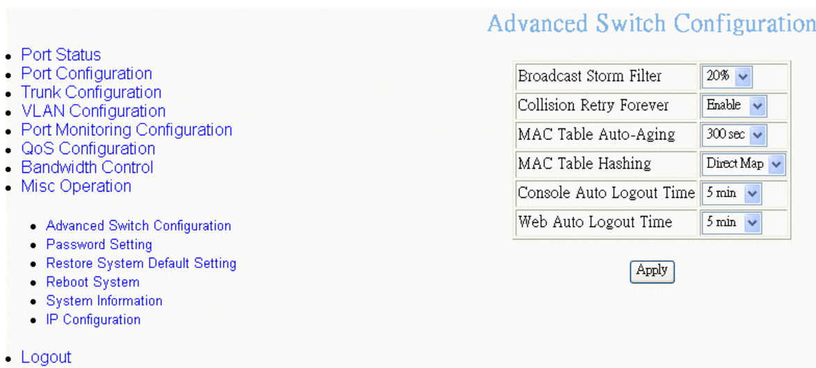
Advance Switch Configuration interface
