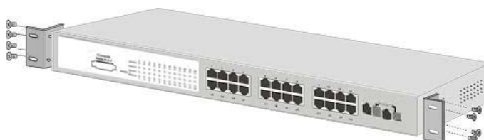
Figure 2-5. Attach mounting brackets with screws
