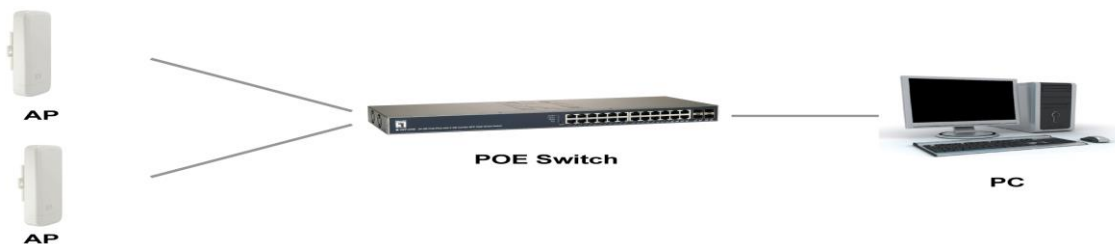
P2 Connection diagram of CPE and PoE
