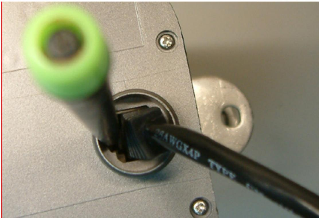
3. At this moment, the screwdriver should compress the RJ45 connector like the picture below inside the WAP-1001.
