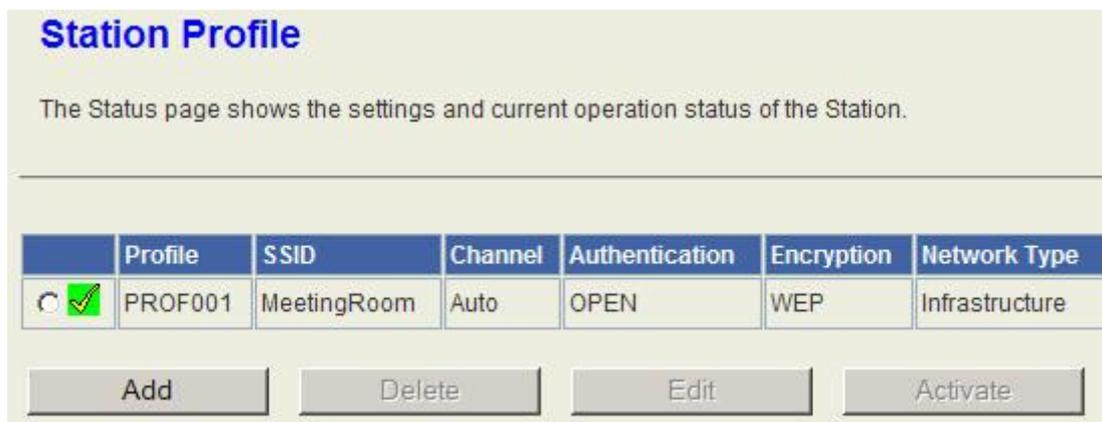
In the first page, you can see the profile list to show the information including Profile name, SSID, Channel, Authentication, Encryption and Network Type. Use four buttons to manage the profile list. The “Add” button is to add a new profile. The “Delete” button is to delete the selected profile. The “Edit” button is to edit the selected profile. The “Activate” button is to enable the selected button, so this device will associate to the AP according to the profile.
