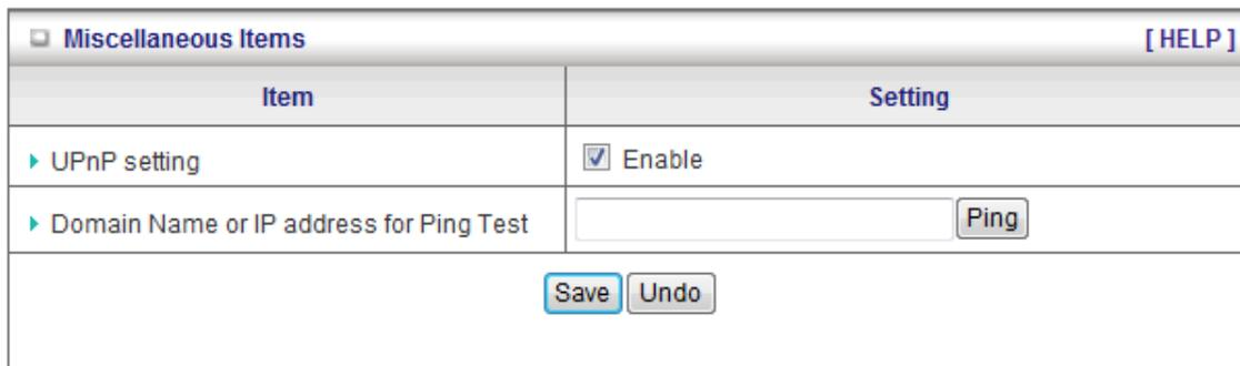
1. **Domain Name or IP address for Ping Test:** Allow you to configure an IP, and ping the device. You can ping a specific IP to test whether it is alive.
